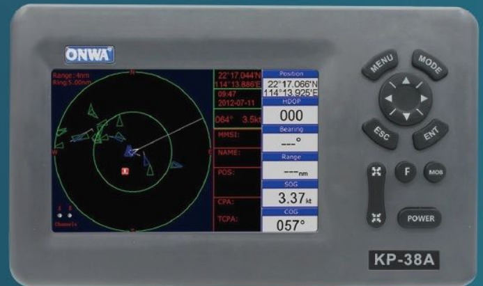
AIS targets on AIS screen
